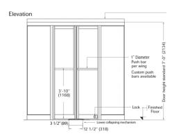
Custom Dimensions are available in almost any size. \* Denotes standard size doors in 7' 0"(2134) height. All other sizes and heights are custom fabricated and finished to suit specific job requirements. IMPORTANT NOTICE: 3 -WING models have a smaller opening width and therefore we recommend that 2 units be considered for in/out traffic flow.
