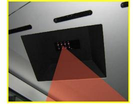
The TOF sensors capture reflected light to create images of the door users. This image is compared to a database of stored images to determine whether there are one or two persons entering or exiting a secured area on a single security authorization. Unauthorized persons are required to exit the door when it reverses on a security violation detection. It prevents unauthorized entry, ensures a safe and secure internal environment for employees and property.
